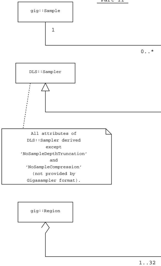
All attributes of DLS::Sampler derived except 'NoSampleDepthTruncation' and 'NoSampleCompression' (not provided by Gigasampler format).
